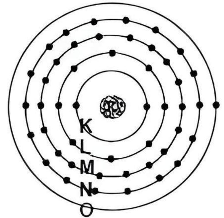
As described in ASTM E1621, X-ray fluorescence (XRF) spectrometry is utilized to determine the presence of metallic and non-metallic elements in solid and liquid samples. The process involves bombarding a sample with high-energy X-rays, which ionize atoms by causing electrons in the inner orbital shells to be ejected into outer shells.
